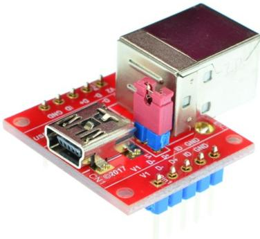
Figure 3: USB-mBF-BF-V1A with headers
