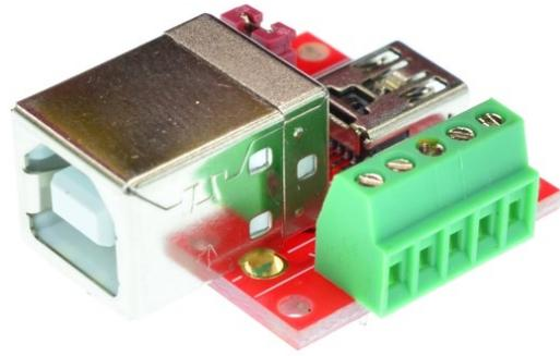
Figure 4: USB-mBF-BF-V1A with terminal blocks
